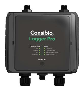
Consibio LoggerPro™ is a modular industrial datalogger and controller capable of collecting and sending sensor data to Consibio Cloud (or self-hosted endpoints) and control actuators in a decentralized setup. All using the newest wireless technologies, completely plug&play.
